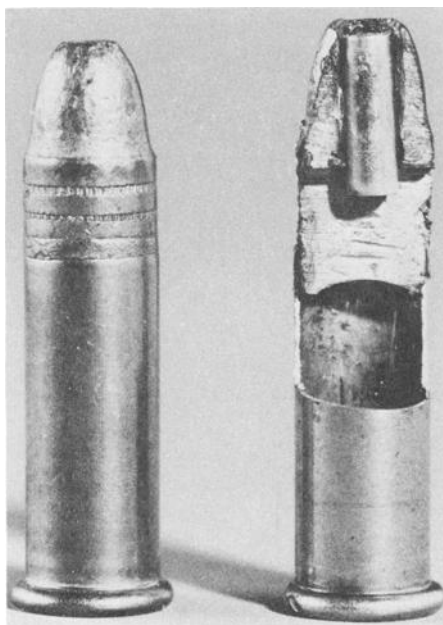
Devastator ammunition: (left) intact bullet and (right) a cross section.
